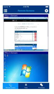
Configuration menu can be displayed / hided by tapping a gear icon in upper right corner:
